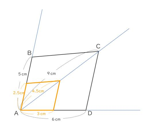
$5 \text{ cm} \times \frac{1}{2} = 2.5 \text{ cm}$   $9 \text{ cm} \times \frac{1}{2} = 4.5 \text{ cm}$   $6 \text{ cm} \times \frac{1}{2} = 3 \text{ cm}$
